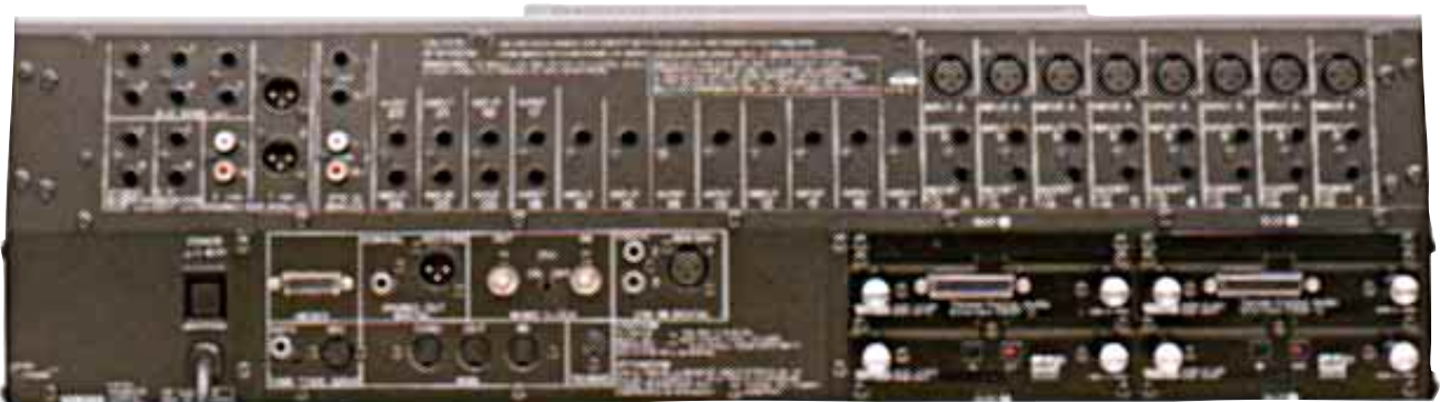
Rear panel of 02R shown with the optional TASCAM & ADAT Interface Cards installed.
